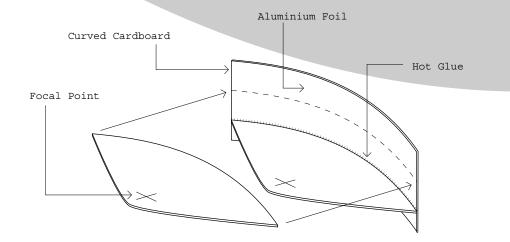
Finally, insert the routers antenna through the focal point cross marks and slide the reflector down the antenna shaft. The reflector is now finished, face it in the desired direction and test.
