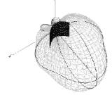
The reflector will change the coverage pattern of your wireless router making it directional rather than omni-directional.
